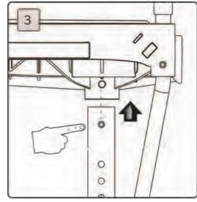
**Step 3** - Attach the Lower Assembly to the Knee Platform by pressing in the silver button on the Height Adjustment Tube and inserting the tube into the socket of the Knee Platform. Tug on the tube to confirm that it is securely locked in.
