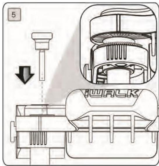
**Step 5** - Before attaching the Thigh Support to the Handle, note that there are raised 'teeth' on the upper surface of each Thigh Support and on the lower surface of the Handle. These teeth must interlock to prevent rotation of the Thigh Supports when the crutch is in use.
