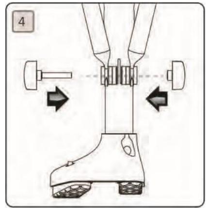
**Step 4** - Position the Clamp so it aligns between the ends of the support tubes. You can use gentle pressure to move the Support Tubes while you rotate the Clamp into position. Gently push the support tube ends and align all 4 holes, then insert the Clamp Bolt through the holes. Thread the nut onto the end of the bolt. Do not tighten completely yet.
