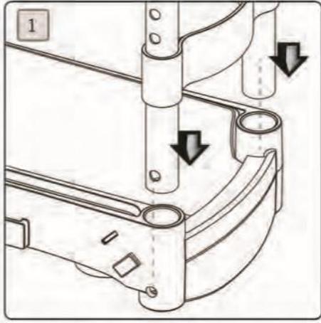
**Step 1** - With the Handle facing forward, insert the tubes of the Upper Assembly into the sockets of the Knee Platform. If the hole at the bottom of the Left tube does not align with the hole in the Knee Platform, rotate the tube until it does.
